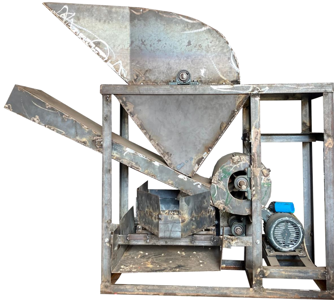
Our V2 peanut sheller prototype. The sheller is capable of processing 120kg of shelled peanuts per hour on a 1.5kW motor. In contrast, a single person can process 0.5 to 1 kg of shelled peanuts per hour by hand.
